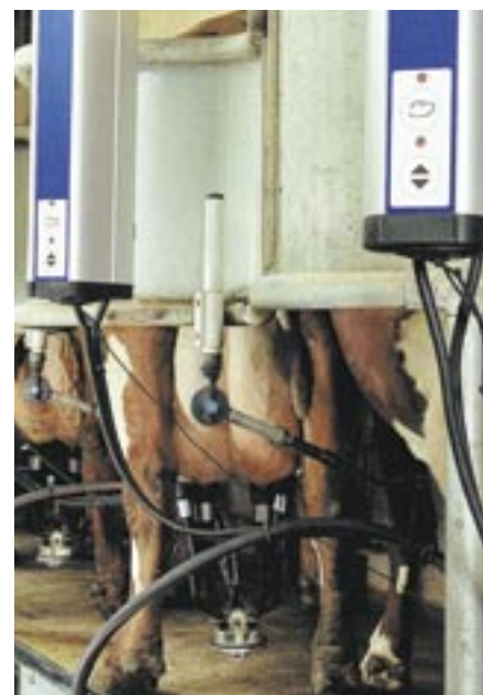
DeLaval milking point MP400 ensures automatic cluster take-off at the right moment.
